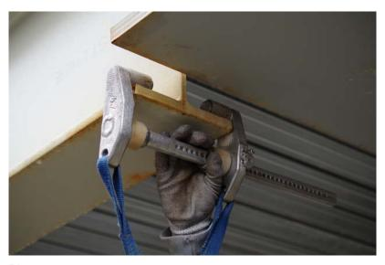
**Photo 2:** First accident: Beam glider at open end of beam (37mm wide gap) [Reconstruction]
