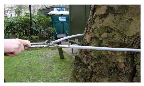
Photo 1: Strop set up as a Primary Anchor. There were four of these together to anchor four ropes.
