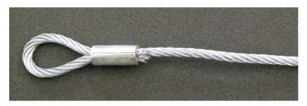
A member working on an oil platform issued a non conformity / improvement opportunity report, after it was noticed that sparks had come from a galvanised wire anchor sling. Since the possibility of causing a spark is obviously to be avoided in any potentially explosive atmosphere the work was stopped. In a safe area, the sparking was replicated by rubbing the wires on a piece of rusty steel.
